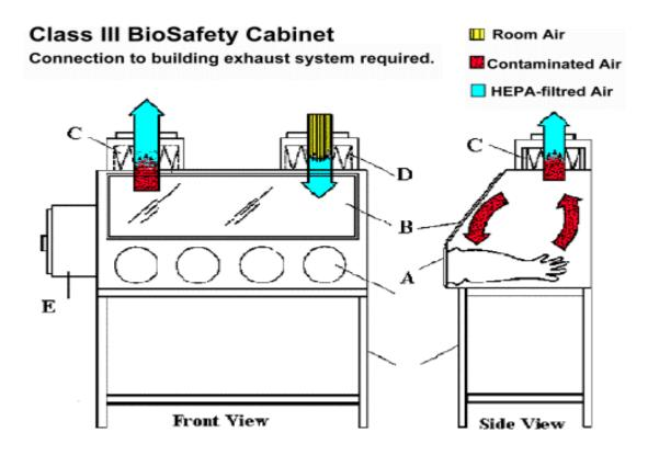
With a Class III BSC, a chemical dunk tank may be installed which would be located beneath the work surface of the BSC with access from above. The cabinet exhaust needs to be hard connected to an independent dedicated exhaust system. The exhaust air must be double HEPA filtered or HEPA filtered and incinerated.
